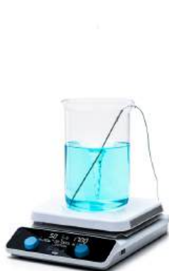
AREC 10 Advance System with Temperature Probe
