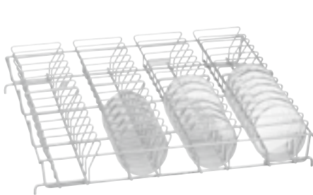
E 137 Insert, for 56 half Petri dishes. • Suitable for 56 half Petri dishes with Ø 100 mm • Equipped with 56 holders, height 70 mm, spacing approx. 26 mm • For use in lower basket • For use with insert E 136 • H 95, W 485, D 445 mm
