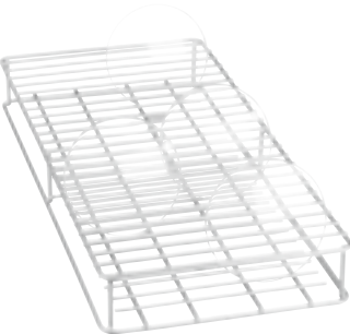
E 402 Insert, for max. 44 watch glasses. • Suitable for 44 watch glasses, Ø 80–125 mm • Equipped with 23 bars spaced 15 mm apart • H 53, W 200, D 445 mm
