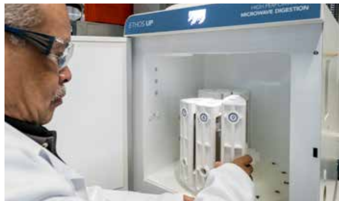
After digestion, the asphalt or construction material is analyzed in this ICP-AES. (Photo by Marco Vellinga)
