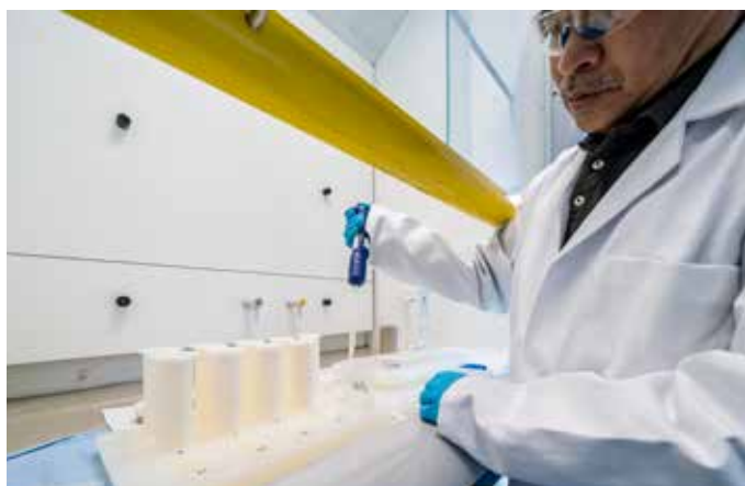
Preparing the vials for digestion in the ETHOS Up high-performance microwave digester. (Photo by Marco Vellinga)
