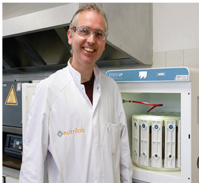
Photo: R&D manager Bart van der Nagel with Milestone's ETHOS Up microwave digestion system with which Nutrilab performs the digestion of samples for ICP-OES element analysis and ICP-MS contaminants analysis.
