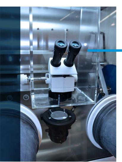
Complete Stereo microscope for the integration in MBRAUN gloveboxes / windows.
