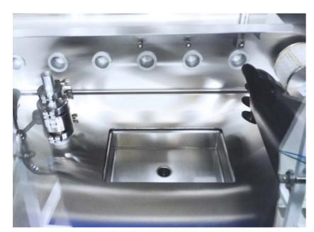
Function: In case of spillages inside the glovebox it facilitates the cleaning process. Available with gas gun for liquids or for gases.
