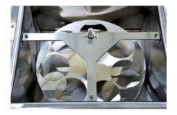
The rotary shelf can accommodate max. 7 bottles (d = 120 mm, h = 250 mm), which are secured by guides from falling over.
